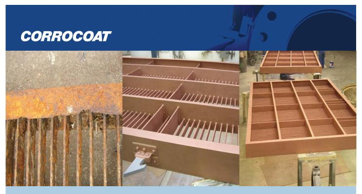
Case study: Coarse water filter screens pro-biofoul anti-foulant
